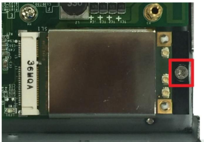
14. Connect antenna cables to the cellular module. There are three antenna connectors on the cellular module: W1 and W3 are for cellular antennas and W2 is for GPS antenna.
