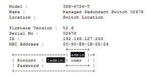
6. The **Main Menu** of the Moxa switch's serial console should appear. (In PComm Terminal Emulator, you can adjust the font by selecting **Font...** from the **Edit** menu.)
