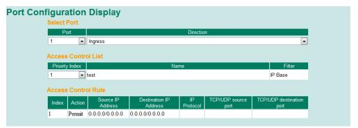
**NOTE** For EDS-828 and PT-7828 series, there are two limitations on ACL settings. Based on the ingress port type of ACL rules, there are two types for the limitation of numbers.
