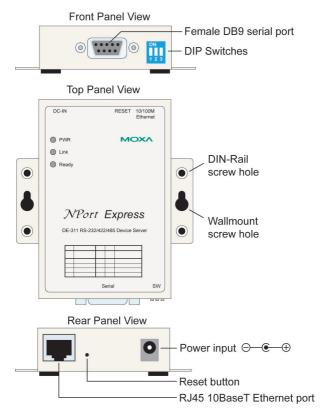
**Reset Button**—Hold the reset button down to erase the password or load the factory defaults, depending on how long the button is held down:
