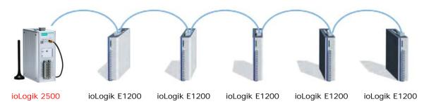
When daisy-chaining an array of devices, the first device in the chain (after the ioLogik 2500) must be connected to the L1 Slave port on the top of the ioLogik 2500 (outlined in red in the diagram).
