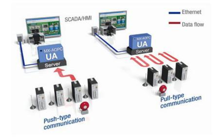
With Moxa's powerful MX-AOPC Server support, communications efficiency between ioLogik 2500-GPRS/HSPA devices and the central SCADA are substantially improved. Moxa's MX-AOPC Server's nonpolling communications architecture supports the standard OPC protocol, but instead of requiring the SCADA to poll edge devices it allows edge devices to actively push communications to the central HMI/SCADA system, empowering the network with real time I/O updates while substantially cutting network overhead.
