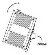
**STEP 3:** The attachment unit should now snap into place along the rail, as shown below.
