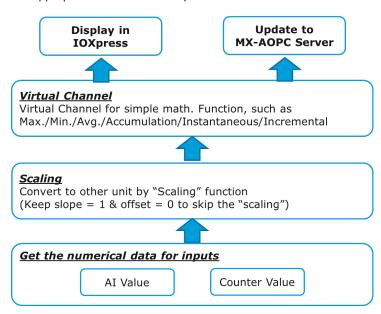
**NOTE** For AI/Counter scaling, configure Scaling on the AI or Counter Configuration panel before selecting operations in the virtual channels.
