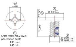
To mount a BXP computer to a wall or cabinet, use two screws on each side for the mounting brackets as shown in the illustration.
